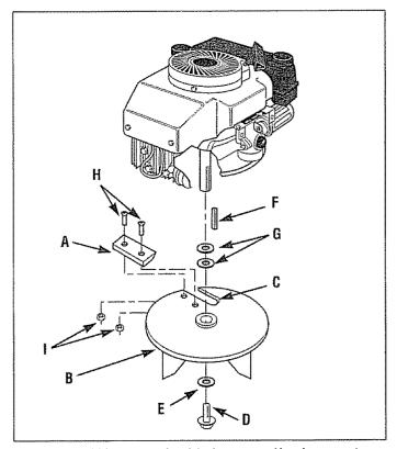
Figure 33: Chipper cutting blade removal/replacement.
